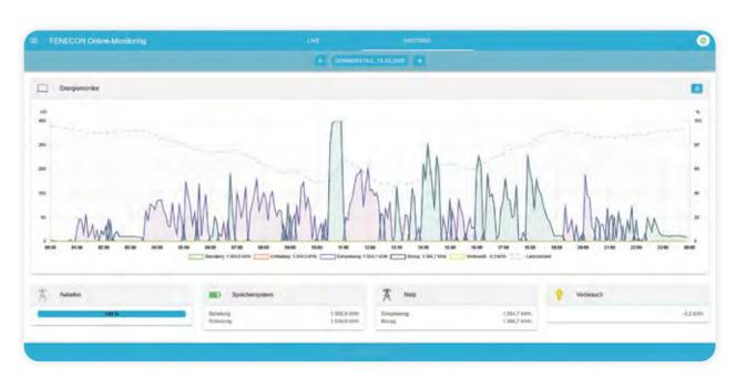
The energy flows are always visible in the Monitoring and can be evaluated at any time. In this case, the system is used for peak shaving. As loads rise and fall dynamically at this industrial site, the system discharges when
