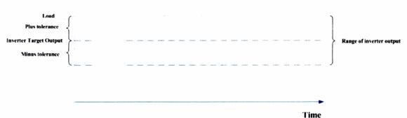
In GMLO mode, the output of inverter is less than load, no electricity feeds into grid
