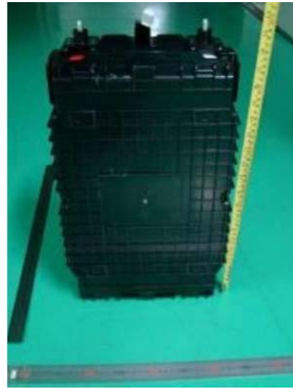
电池/ Battery ( C12_4SI 12,8V 200Ah 2560Wh )
